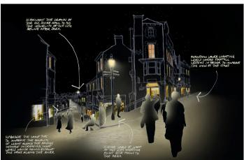
Our recommendations included upgrading all streetlighting, with delineation through colour temperature of primary and secondary roads; illuminating the city's bridges; and creating an events infrastructure.
